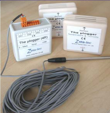
Data loggers used to collect temperature and humidity data for condensation cases.
