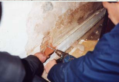
Taking brick samples from a wall for laboratory analysis
